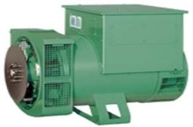
**ALTERNATOR**--Brushless, self-exciting, self-regulation, screen- protected, Drip proof rated in Accordance with IEC60034. Voltage regulation maintained within ±0.5% from no load to full load. Between 0.8 lagging and unity. All standard voltages available.
